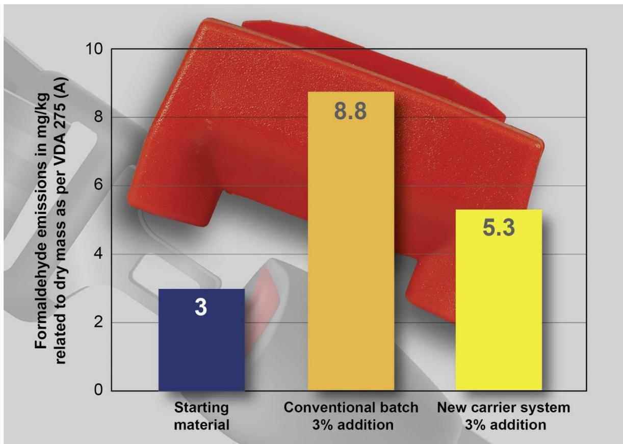
*With the new optimized masterbatches from Tosaf Color Service, the formaldehyde emission from POM components remains at a low level. © Tosaf*
