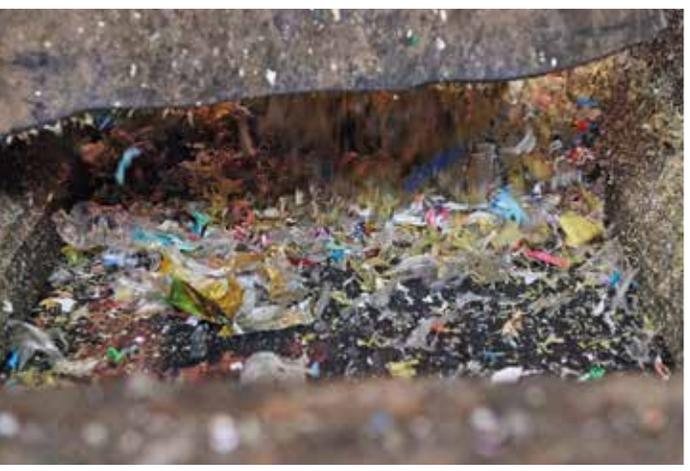
The raw material arrives at InnoPlastics in highly varying quality, pressed into balls. This material is shredded, washed repeatedly and dried extensively in various machines before it is extruded into new regranulate. As participants in an energy-saving program, we take care that no energy is wasted during the recycling process.
